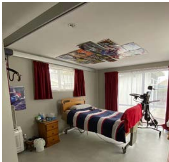
Image 1: new bedroom layout with overhead hoist, profiling adjustable bed and standing frame
