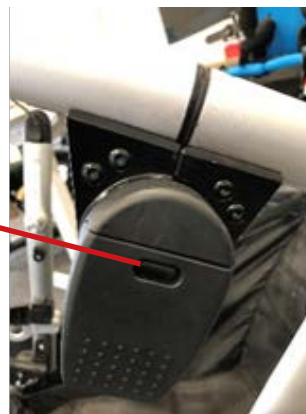
T Bolt is not damaged
