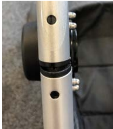
Gap at the folding joint and locking disc protruding
