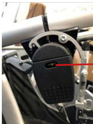
Damaged T Bolt is visible through the folding tab
