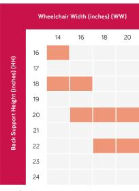
Adapta<sup>3</sup> Back Supports have an additional 2" of padding length to accommodate adjustments.
