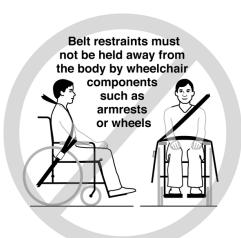
Figure 3a - Improper positioning of pelvic-belt restraints over wheelchair supports. Figure 3b - Proper routing and positioning of belt restraints on the wheelchair occupant.
