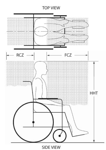
NOTES: The rear clear zone is measured from the rearmost point on an occupant's head. The front clear zone is measured from the front most point on an occupant's head. Seated head height (HHT) ranges from about 1200mm for a small adult female to about 1550mm for a tall adult male.
