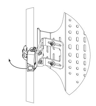
**10.** Evenly torque both clamp fasteners to 5Nm. Check both fasteners are tight.
